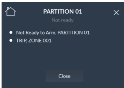
Figure 29: Partition Failed to Arm Screen
